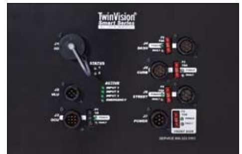
Vehicle Health Monitoring Panel
